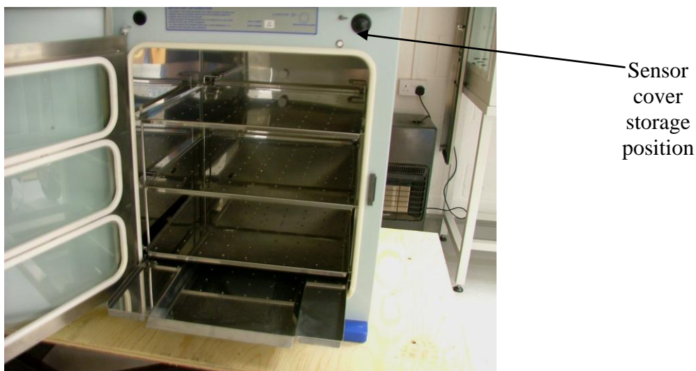
Figure 5. Water tray (bottom) partly removed.
